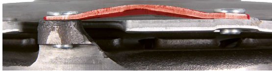
Verbogene Tangentialblatfeder Bent tangential leaf spring
