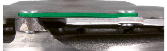
Korrekte Tangentialblatfeder Correct tangential leaf spring
