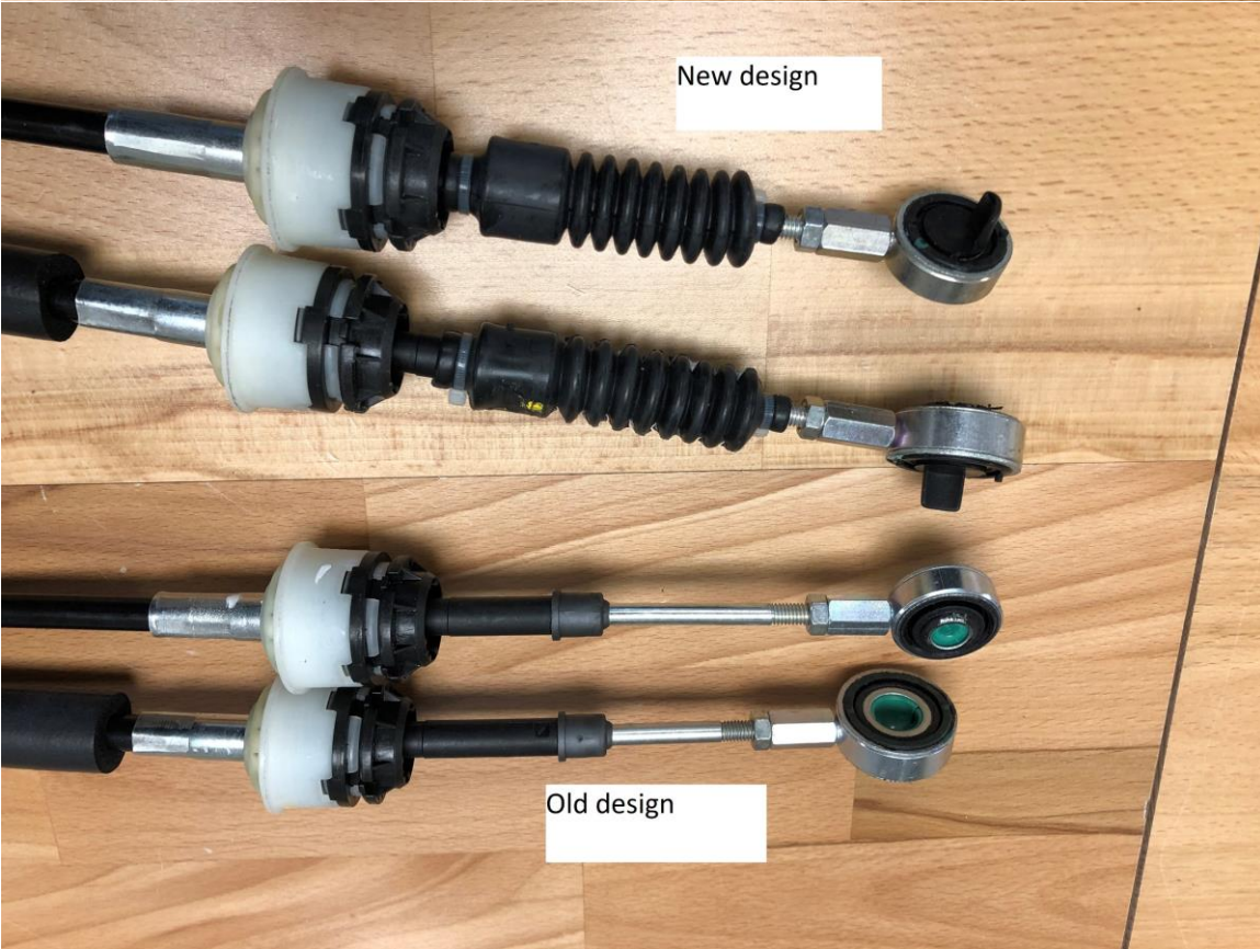
New cable design 55247553 improved by fiat from 02/07/2012 but can be used retroactively on all cars and therefore replaces 55231412
