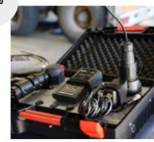
8. With the trailer test case (article number: 95980571), the function of the combination rearlights can be tested once installation is complete. The benefit: The test case enables both the assignment of the trailer socket and the light function of the trailer to be verified by just one person.
