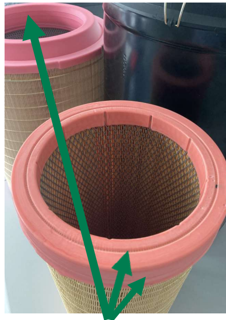
cover secondary element and inner side main element should be greased
